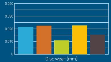
Ultimate C and A series have been tested in low steel formulation in comparison with antimony trisulphide. Ultimate 45-7 in comparison with molybdenum disulfide. The total amount of lubricant in the material is 5%vol. The tests have been performed on a full-scale dynamometer.
