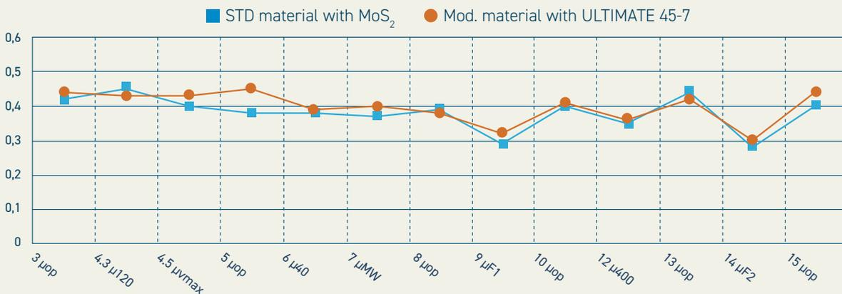
AK-Master Comparative dyno tests show that ULTIMATE is a valid alternative to common lubricants such as Sb<sub>2</sub>S<sub>3</sub> and MoS<sub>2</sub>
